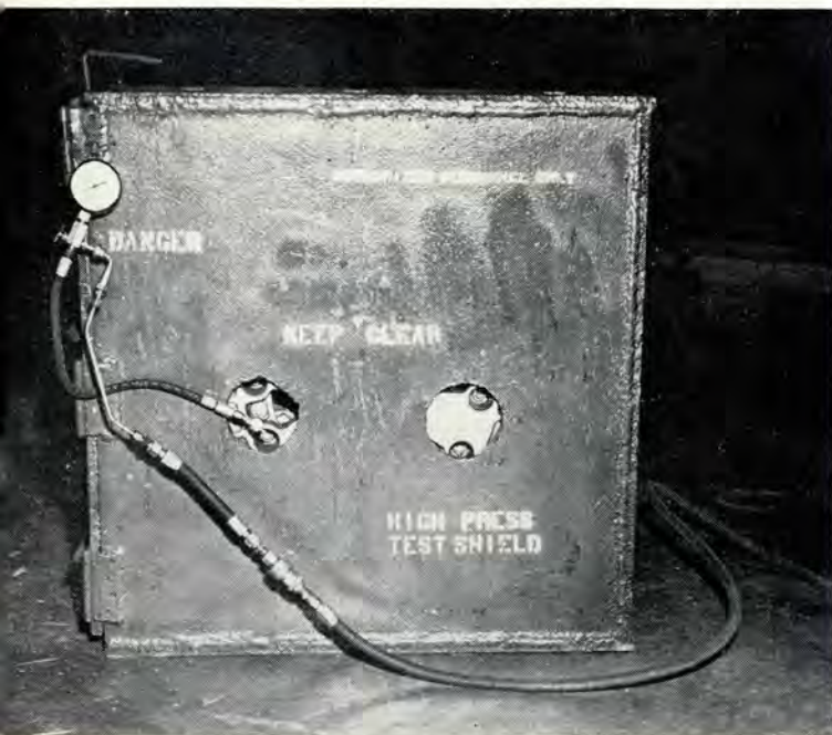
Another type of tire cage guard referred to in T. O. 4T-1-2. This cage and remote reading pressure gage offer maximum protection.
